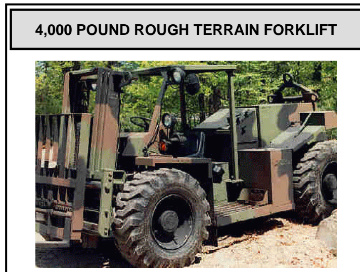
Figure J-4. 4,000 Pound Rough Terrain Forklift
