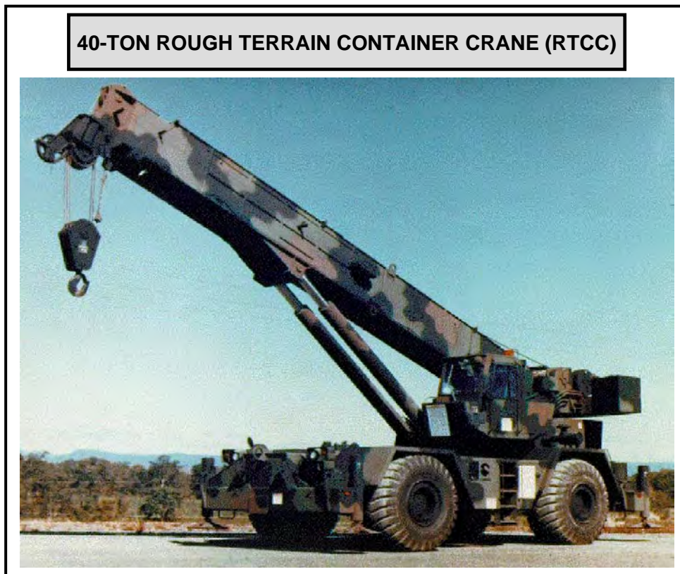
Figure J-3. 40-Ton Rough Terrain Container Crane
