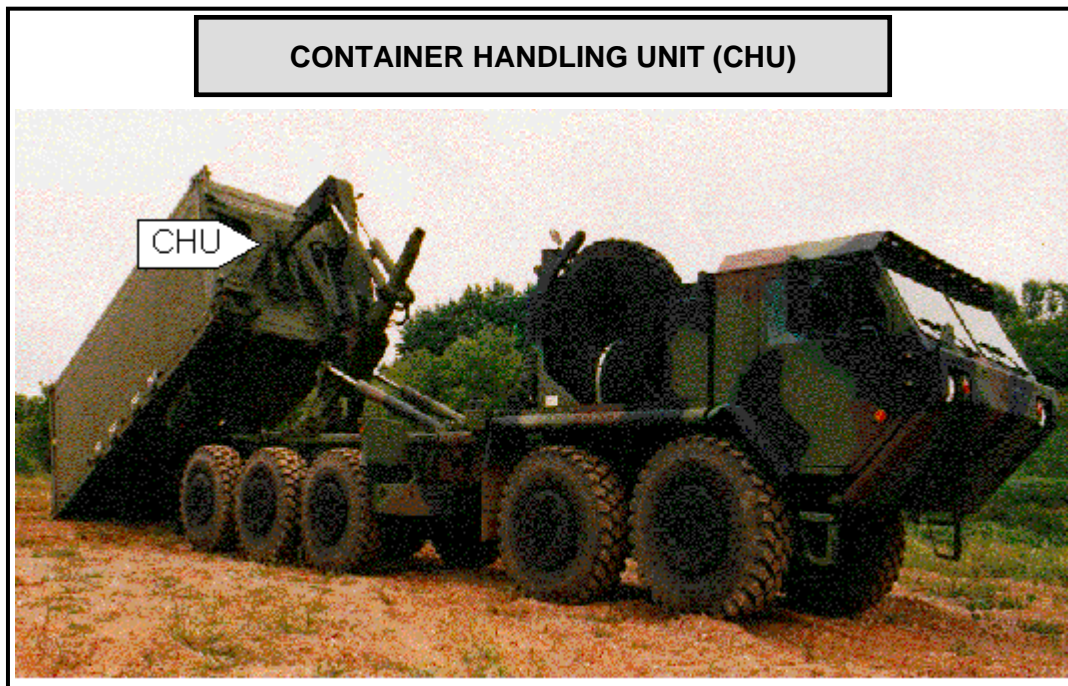
Figure J-7. Container Handling Unit (CHU)
