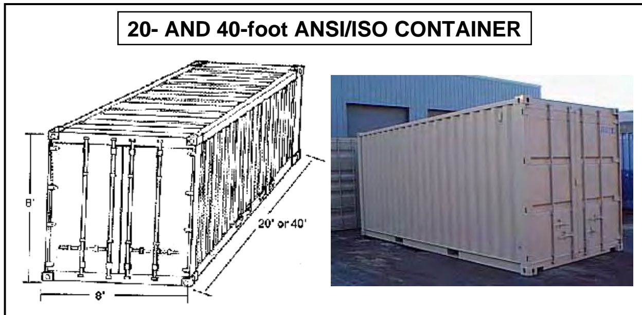
Figure J-9. Common Intermodal Container
